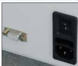
SUB D9, electric supply
