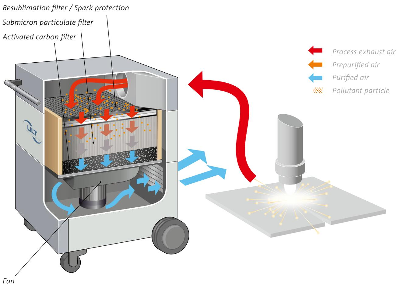
Functional principle of saturation filter units
