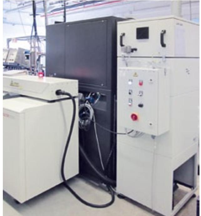
*Laser welding system with integrated extraction and filtration system*
