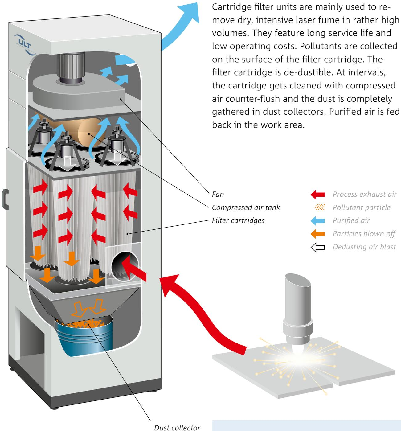
*Functional principle of cartridge filter units*
