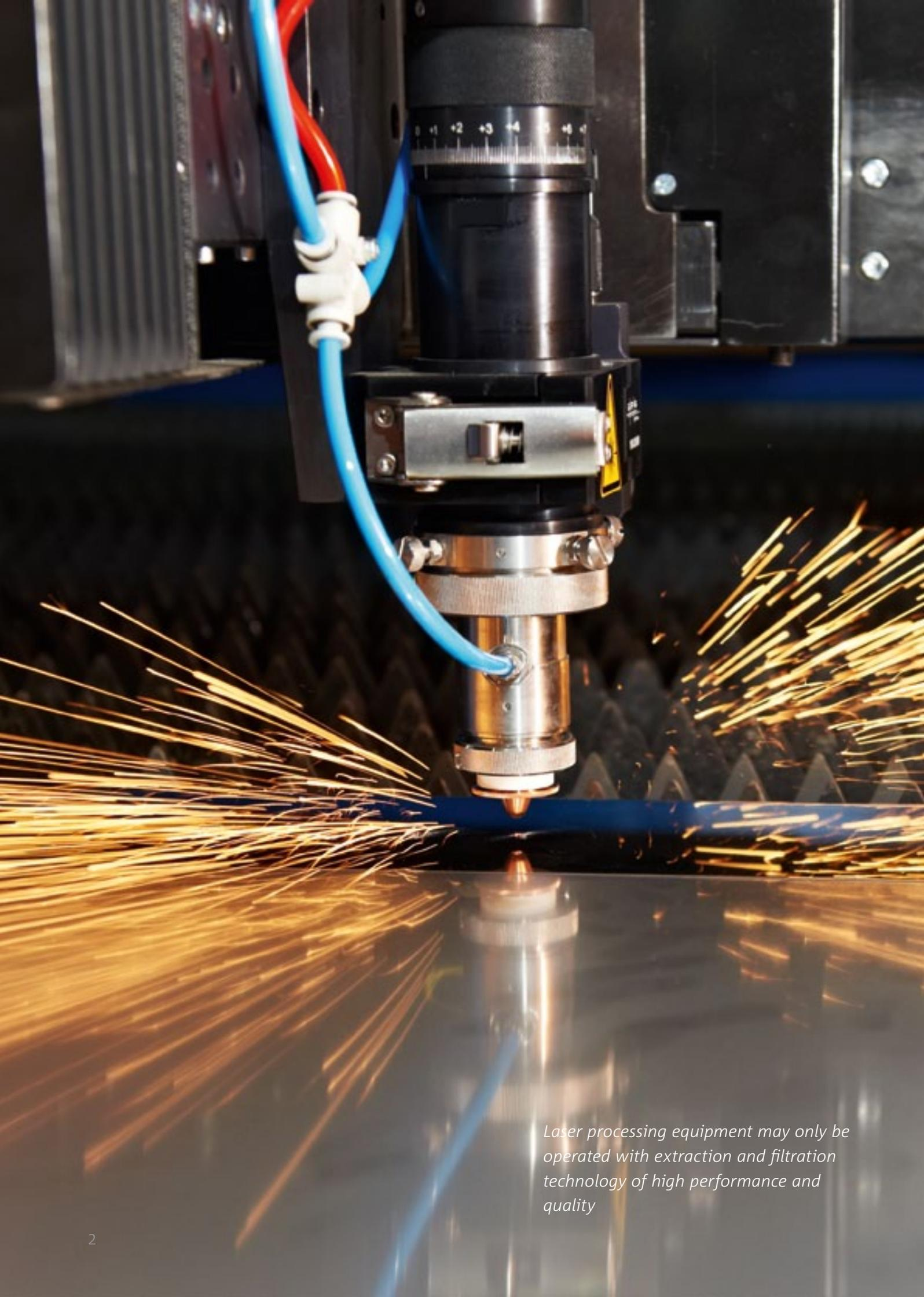
*Laser processing equipment may only be operated with extraction and filtration technology of high performance and quality*
