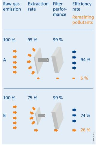
Impact of the extraction rate on efficiency
