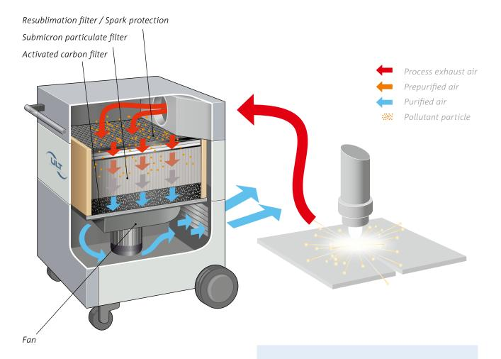
Functional principle of saturation filter units
