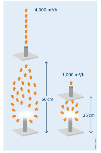
*Impact of the distance of the collecting element on the required air capacity*
